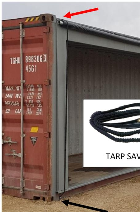
The Tarp Saver Cord will be installed on both ends of the container. It needs to wrap around the bottom of the hoods and to the container. See Black Arrow. The top of the Tarp Saver Cord will be mounted to the top of the container. See Red Arrow. They should be mounted over the hoods. That way they do not interfere with the opening. Some tension needs to be applied to the Tarp Saver Cord in order to keep the tarp and Roll Tube from swinging in the wind.
